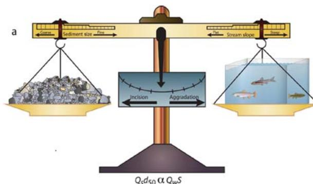
Figure 7: Lane's Balance showing the conceptual response to changes in slope, sediment input, discharge, and sediment size from Pollock, 2014.
