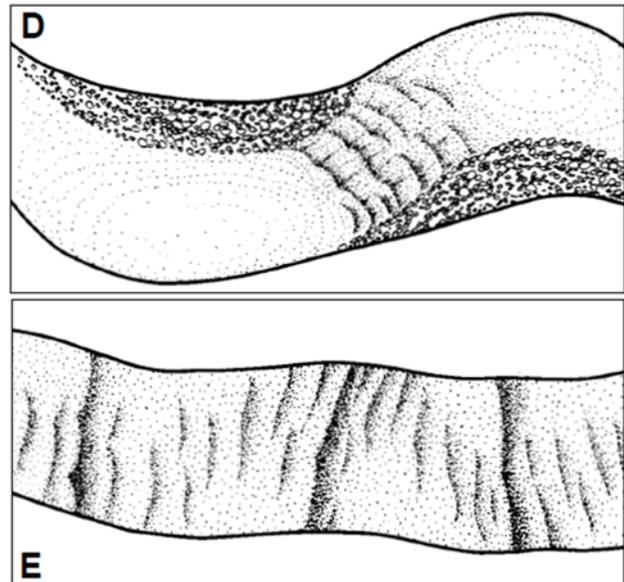
Figure 2: An idealized diagram of a pool-riffle (D) and dune-ripple (E) channel from Montgomery and Buffington, 1997
