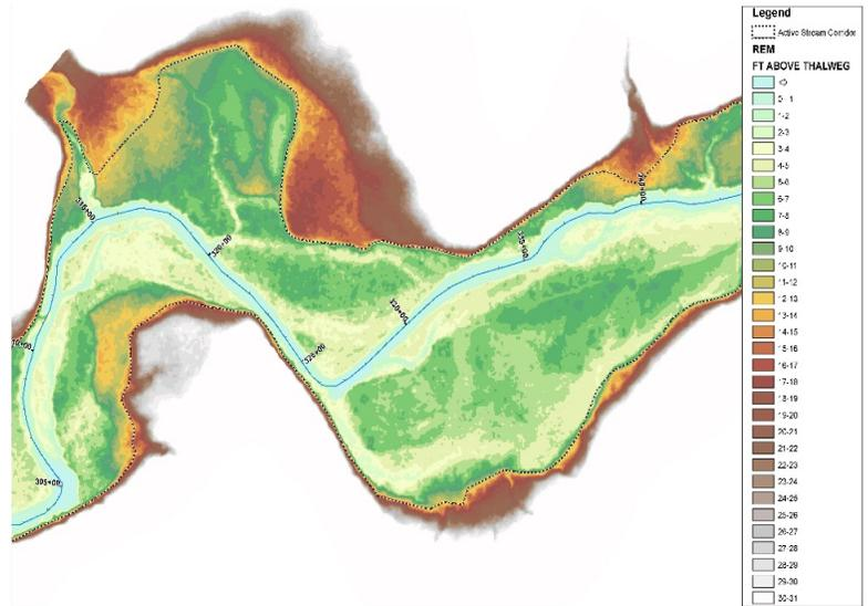
Figure 3: An example of the relative elevation model (REM) used to delineate the active stream corridor and in turn the width for unit stream power calculations.
