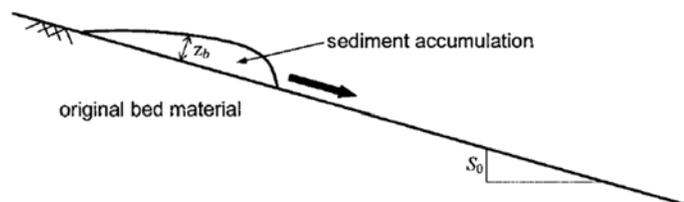
Figure 8: Illustration of a sediment influx moving as a wave along a slope from Greiman et. al, 2006.
