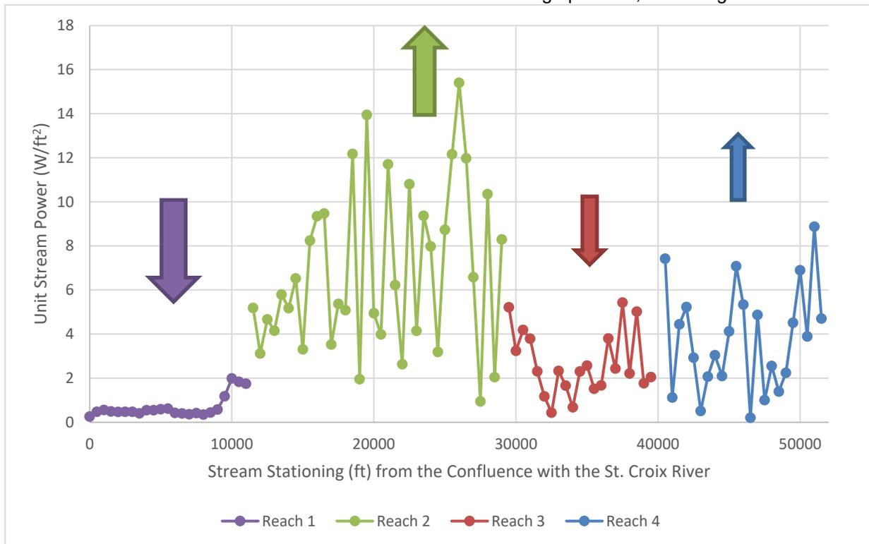
Figure 4: A plot of unit stream power along the study reach of the Kinnickinnic River. The different colors represent the reach breaks within the study reach. The arrows indicate relative change and magnitude compared to adjacent reaches.
