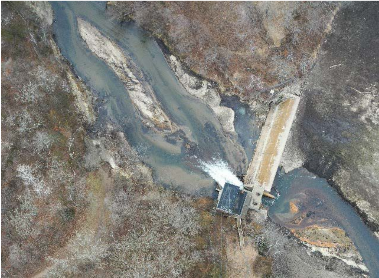
Figure 4: Drone image collected on 12/11 above the Powell Falls dam showing bar development immediately downstream.
