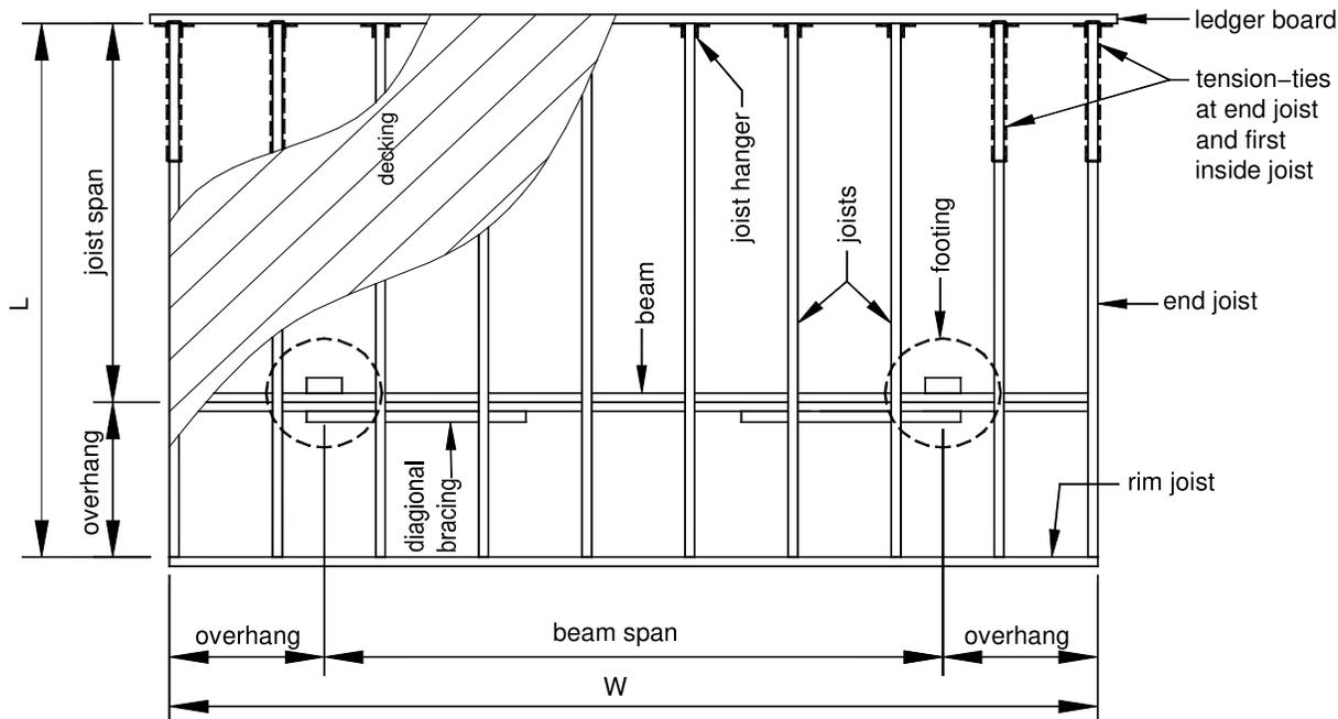
**Decking:**     2x4     2x6     five-quarter board     wood-plastic composite (per ASTM D 7032)
